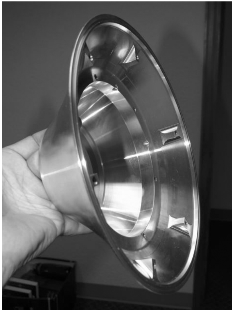
Fig. 2. The lightweight mirror before diamond turning and (for the interior) black anodizing. This size of mirror was chosen to provide 0.1% photometry, within an hour's integration time and a 1^\circ \times 1^\circ sky bin, at about 90^\circ elongation from the Sun, at 1 AU.
