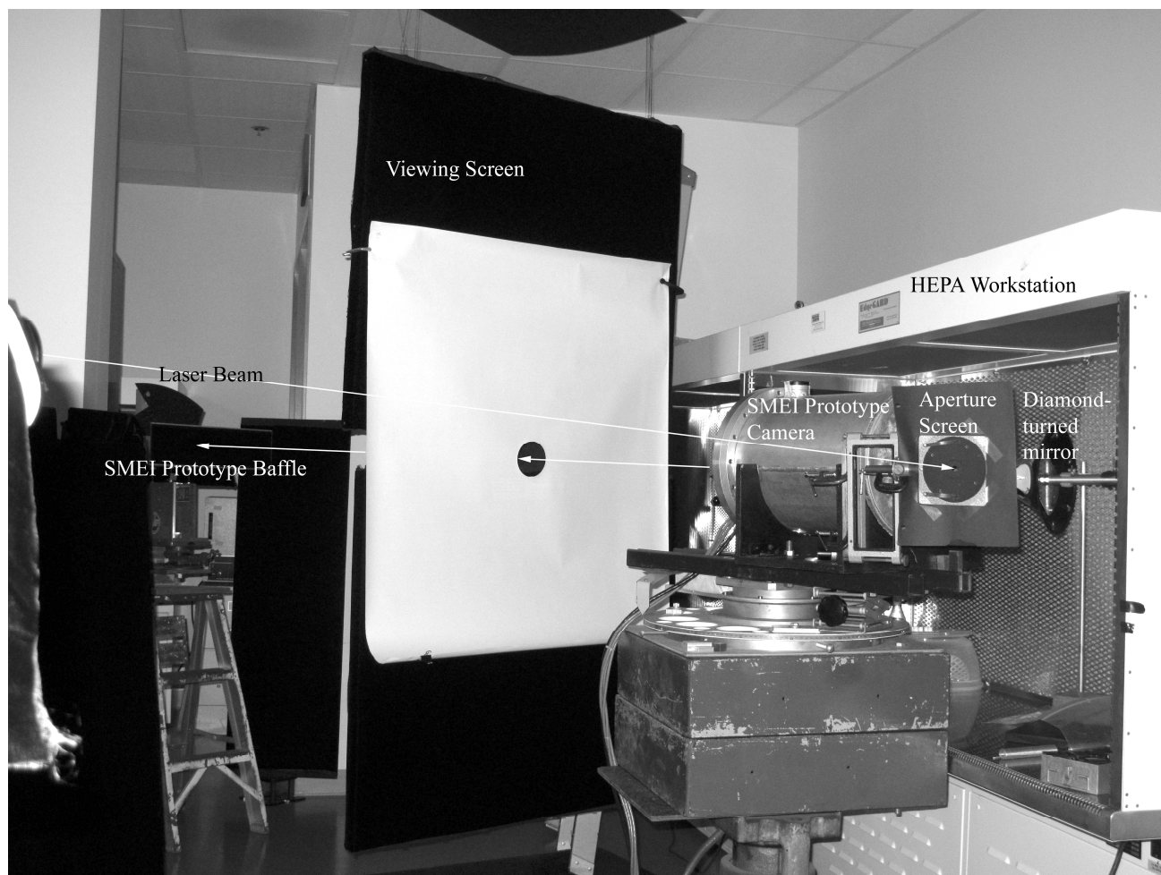
Fig. 5. Photograph of the clean room setup used for the measurements presented here. A specular-reflected laser beam is drawn in to highlight the light's path. Light scattered by more than about 2^\circ , out to about 20^\circ becomes visible on the white paper placed upon the Viewing Screen, where it can then be photographed by a conventional digital camera or photometrically recorded using the SMEI Prototype Camera.
