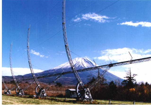
Fig. 3. STELab IPS radio array (one of four now operating) near Mt. Fuji. The arrays used singly measure scintillation intensity (or g-value) for about 50 radio sources each day. Scintillation signals cross-correlated between arrays give a robust IPS velocity determination.
