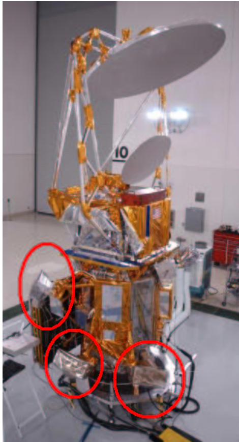
Figure 2. Coriolis spacecraft with the Solar Mass Ejection Imager (SMEI) instrument on board prior to Vandenberg launch. Three instrument camera baffles (circled in red) are seen on the lower portion of the spacecraft.
