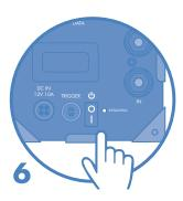
Turn on the camera. Wait 10 seconds before turning the computer on. When the LED on the back of the camera turns off, the camera is ready to image.
