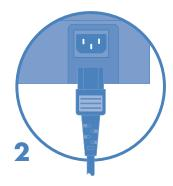
Connect the power cord to the power supply. Plug the power cord into a wall outlet. Plug the power supply into the camera.
