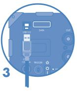
Plug the USB 3.0 cable into the camera. This camera is not compatible with USB 2.
