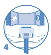
Connect the power supply to the camera head's POWER connector. Secure the power supply by tightening the side screws to the camera head.
