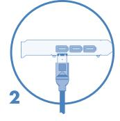
Connect the data cable to the IEEE-1394 card connector. Be sure to connect the cable in the proper orientation.
