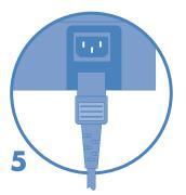
Connect the power cord to the power supply. Plug the power cord into a wall outlet.
