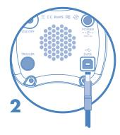
Connect the data cable to the DATA connector on the camera head. Connect the data cable to a UBS port on installed card. Do not connect the cable to any other port.
