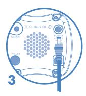
Connect the power supply to the camera's POWER connector and plug the other end of the power supply in an electrical wall outlet.
