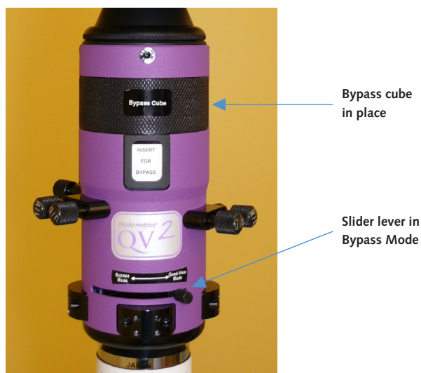
Figure 14. The QV2 with the slider lever in the Bypass Mode position.
