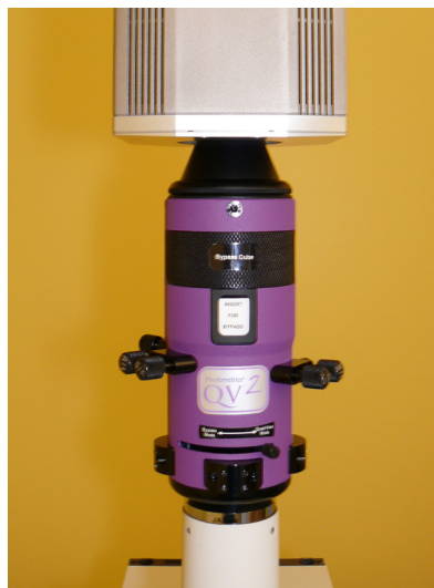
Figure 2. The QV2/camera combination mounted on the top port of the microscope.
