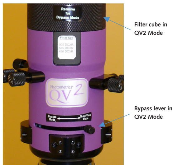
Figure 3. The QV2 with the bypass lever in the QV2 Mode position.
