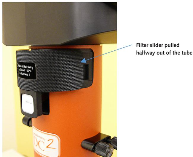
**Figure 2.** Filter cube in Bypass Mode position.
